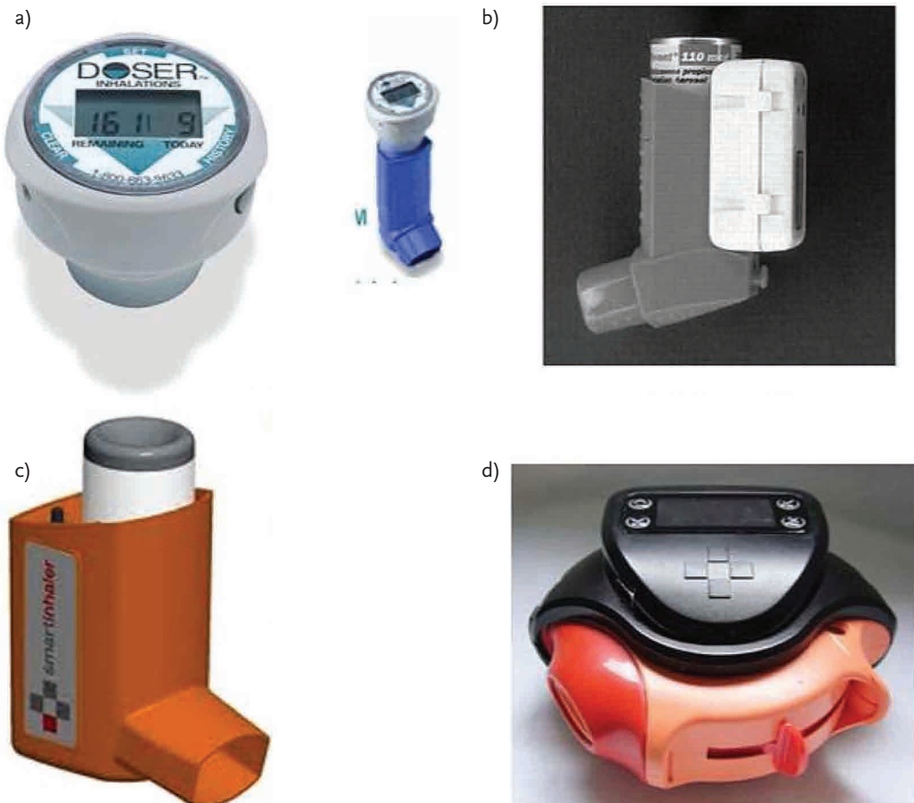
Figure 1 Electronic adherence monitoring devices suitable for use in clinical practice and research. a) Doser, b) MDILog, c) Smartinhaler and d) SmartDisk.
